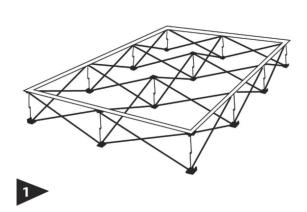
Assemble frame and lay flat on its back. Remove existing graphic.
