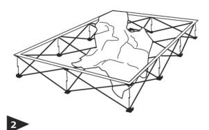
Starting at one corner, attach velcro on the graphic to velcro on the frame.
