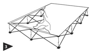
Work in a continuous direction around the frame attach the rest of the graphic.
